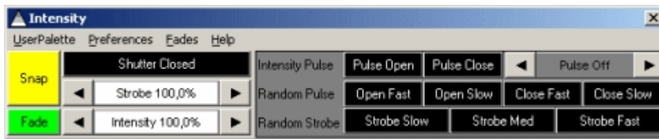
Example MAC500/Roboscan 918 intensity control displaying special functions
